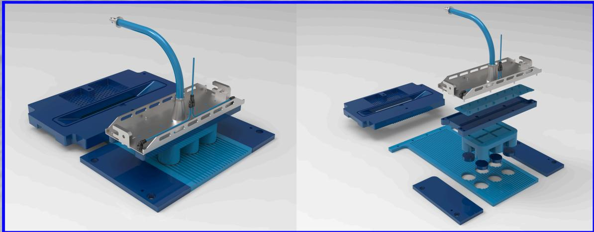
PIASTRA DI FORMATURA TIPO GRILL CON ESPULSORE
